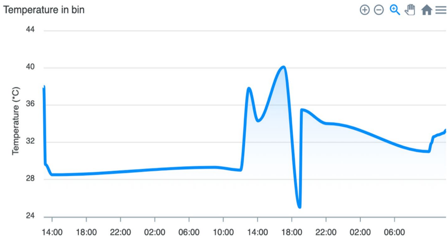
Fig. 5 A time-series graph of the data generated from the smart bin constructed using Javascript libraries from ApexCharts.js. Top–Bottom: Garbage fill level in cms, Temperature in degrees Celsius, Humidity in percentage
